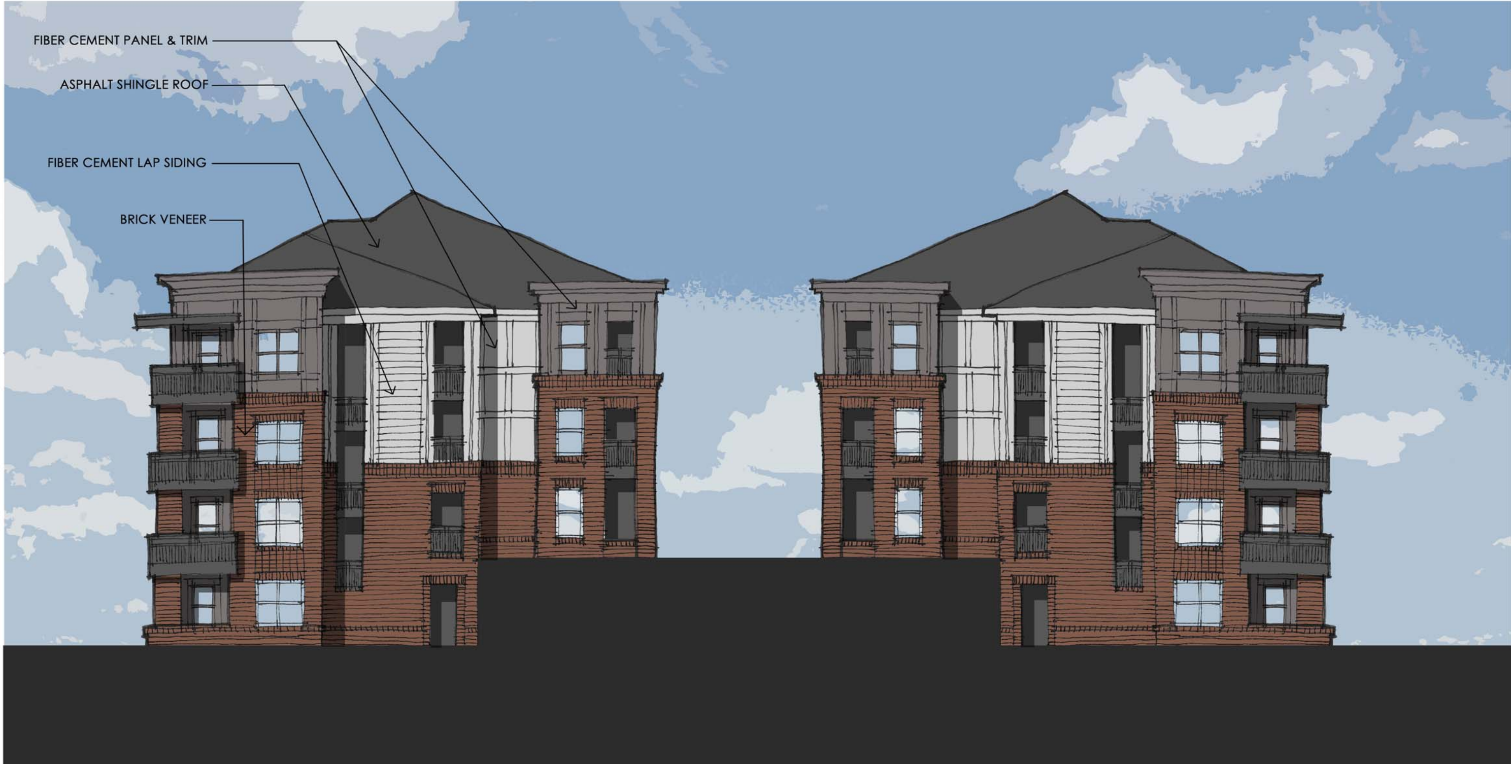
TYPICAL BUILDING SIDE ELEVATIONS
