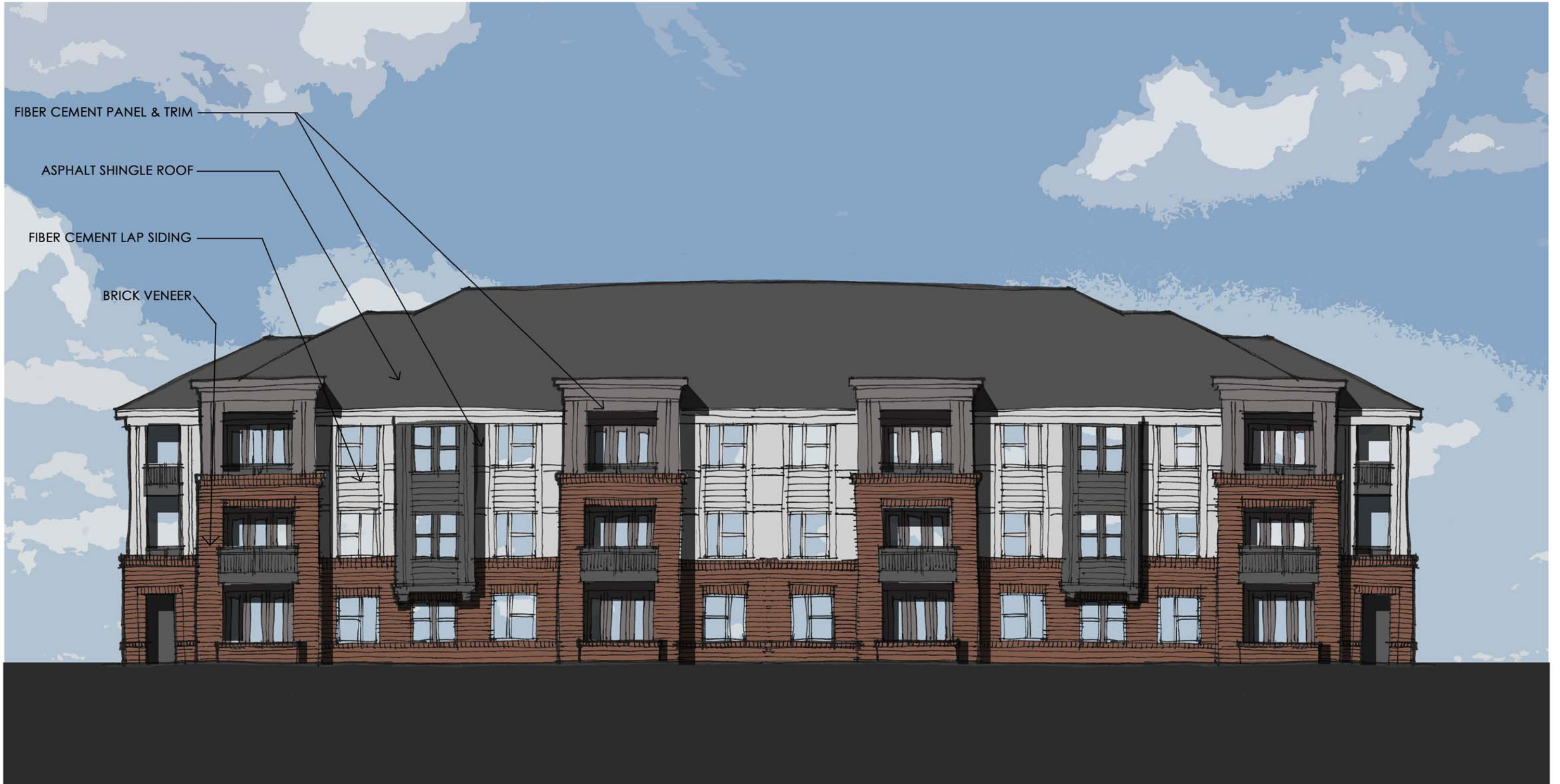
TYPICAL BUILDING BACK ELEVATION
